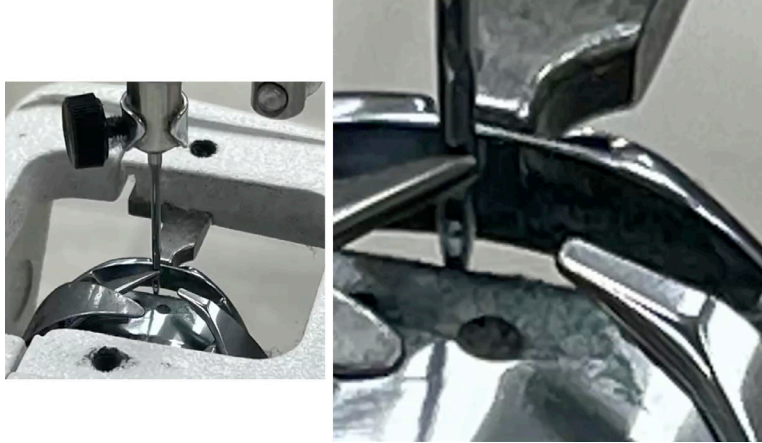
Figure 2 - Proper Timing Hook Position
