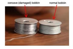
A bobbin can also have a "sloppy" wind if thread jumps out of the tension discs on the winder or if the tension is set too loose. A bobbin is too loosly wound if you can easily push your fingernail into the threads. Be sure the pigtail guide is set to the left of the tension disc, to avoid the thread from jumping out of the discs while winding.
